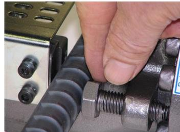
**WARNING:** Failure to correctly set the stopper will result in excessive wear of cutter blocks and **may cause cut end to fly out**. This may lead to piston and cylinder damage.
