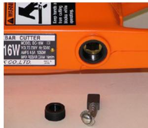
*CARE:* Worn brushes will result in power loss; cause the motor to run hot and irreparably damage the armature.
