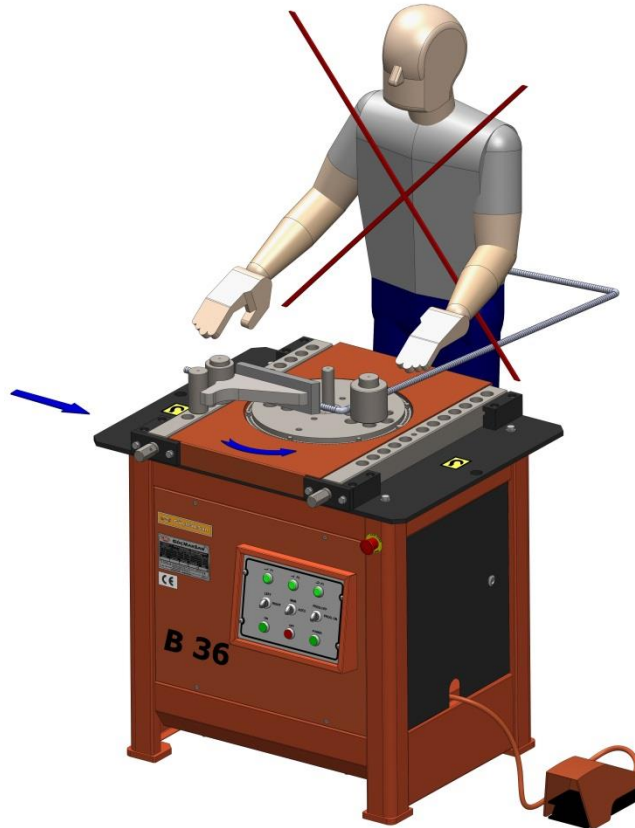
Figure 7: Wrong positioning of the person making bend
